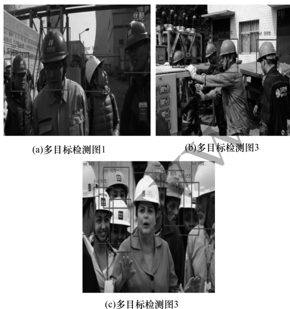
图9 多目标下mobileNet-SSD的检测部分结果展示 Fig.9 shows the results of the detection part of mobileNet-SSD under multiple targets
